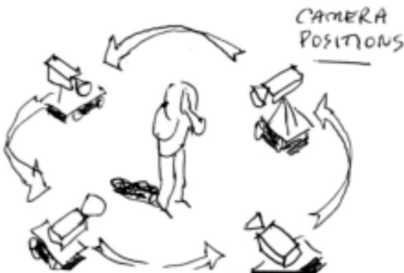
**ARCING** (the camera is moved in a left to right curve where the subject remains in the center.)
